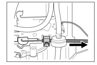
4. Pull the throttle control back to the full throttle position and check that the choke is no longer activated.
